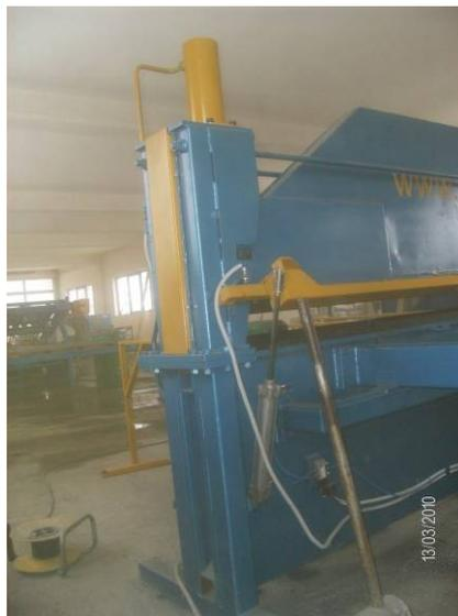
Bending cycle runs according to the given program until the whole panel processing is finished. The press function is based on hydraulic principle. It is powered by the 5.5 kW hydro-aggregate. Raising and lowering of the beam is propelled by hydro-cylinders  $\Phi 125 \times 120$  that are positioned at the beam ends.
