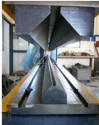
Bending is done by the mean of three wires (which are identified by their axial distance which is less than the others). Middle of those three wires is positioned in the tool using the guide and then the upper beam lowers down. Command for bending is given by the foot pedal.
